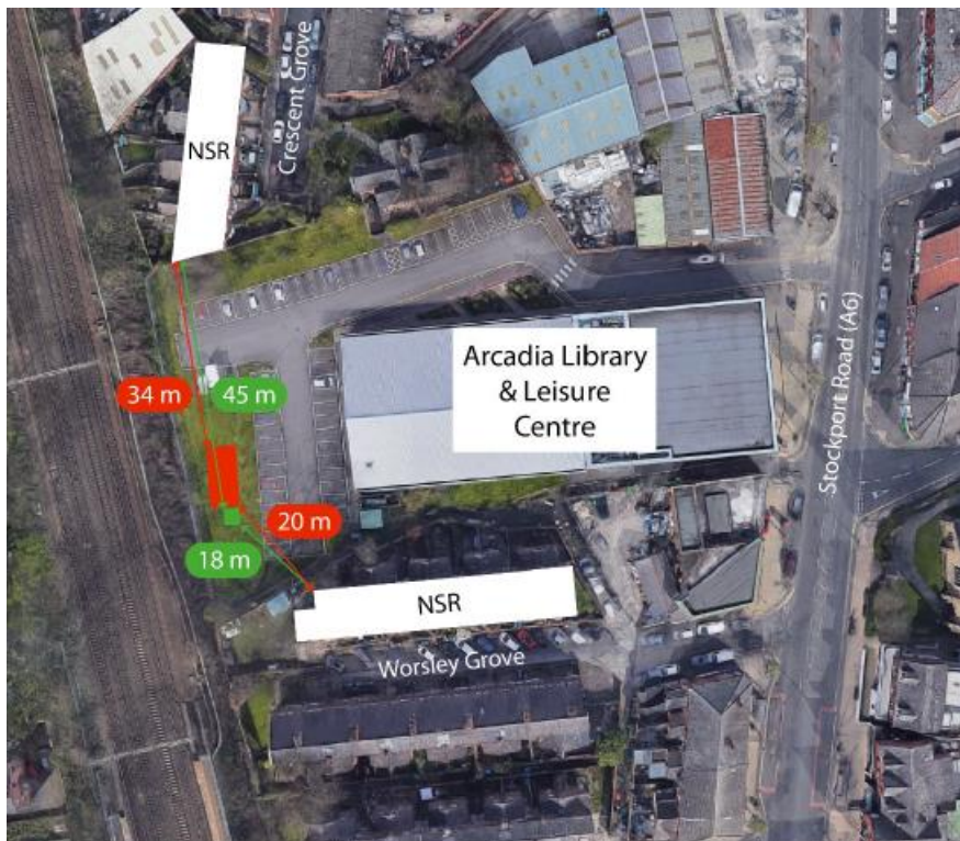
Figure 1: Identified nearest / most exposed NSR properties to the new plant equipment location on the site (ASHP's enclosure location indicated by red rectangle; Battery container location indicated by green square)
