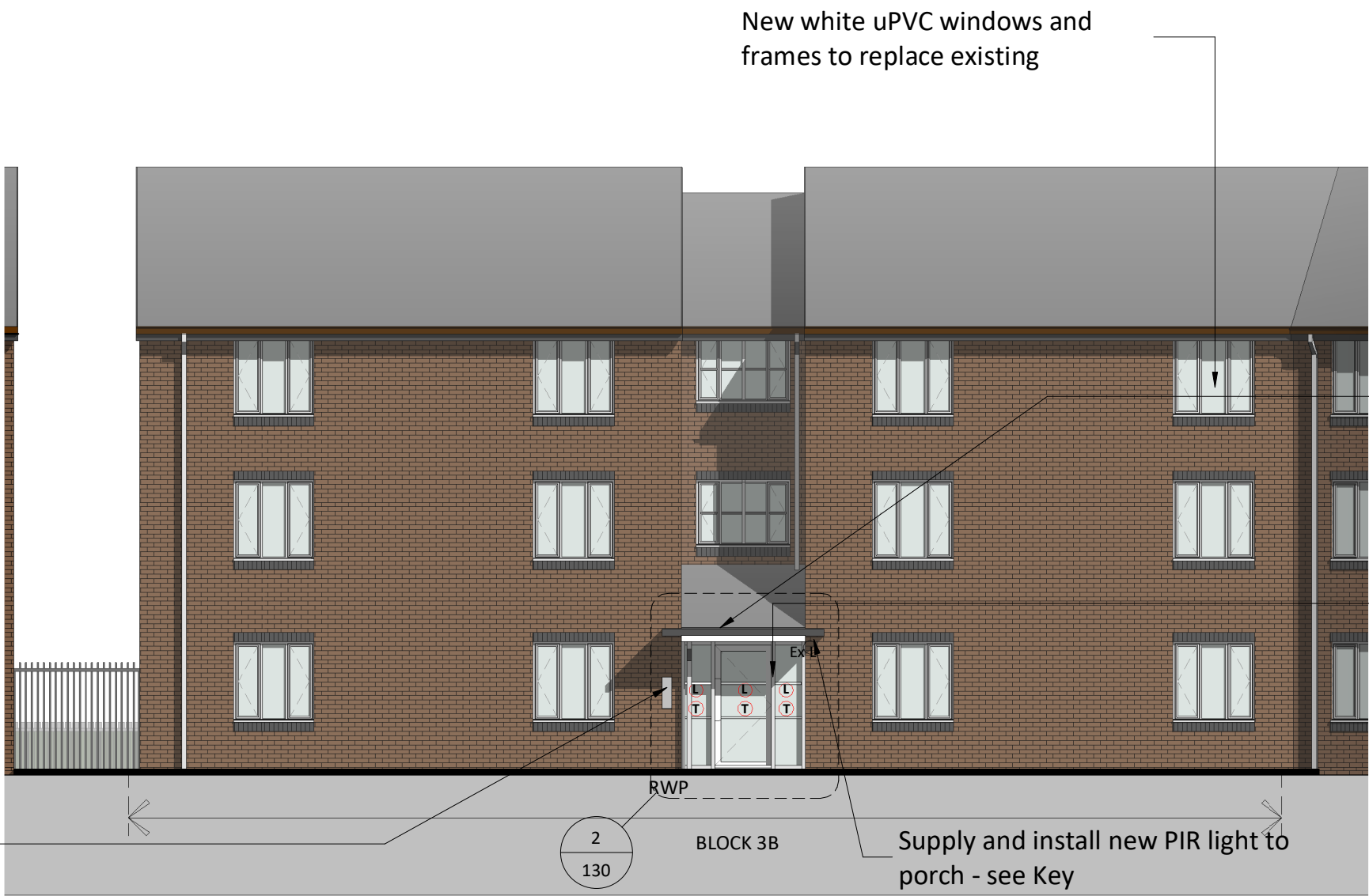
Block 3B - East (Front) Elevation New Works 1 : 100
