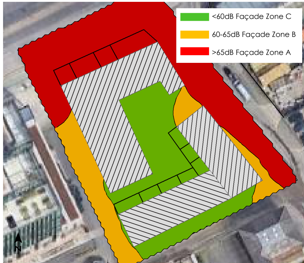
Sound map indicating the external daytime L_{Aeq,16hour} environmental sound levels at 2 nd floor level (7.5m)
