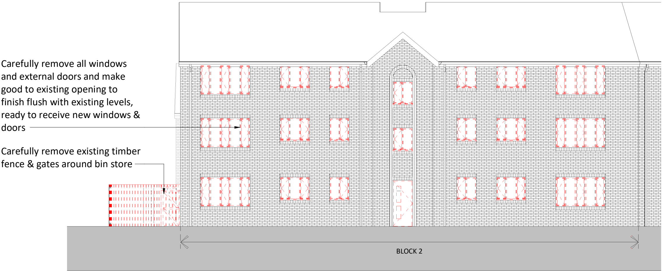
Block 2 - West (Rear) Elevation Clearance 1 : 100
