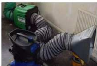
Filtrated mobile dust control unit.
