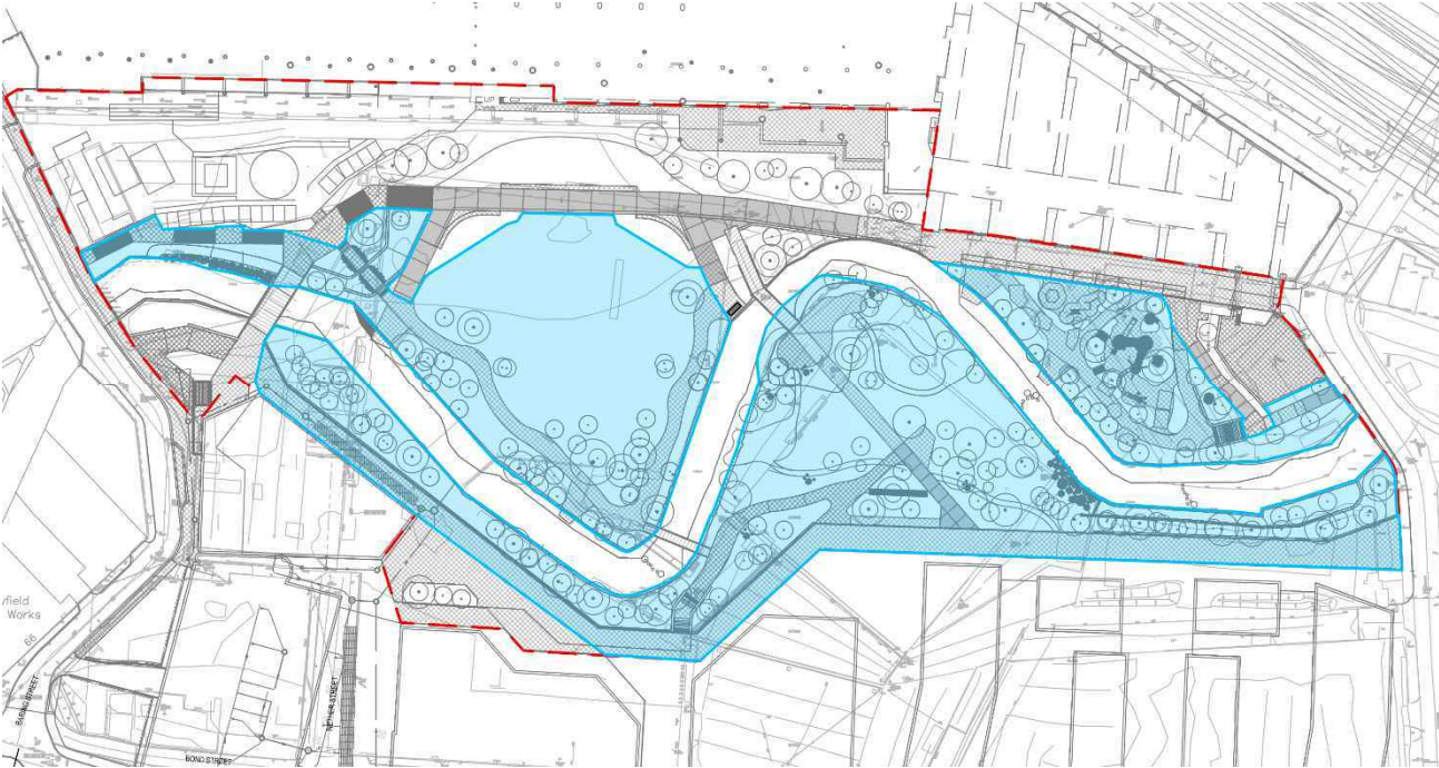
Figure 7-2 Areas drained via overland flow/infiltration
