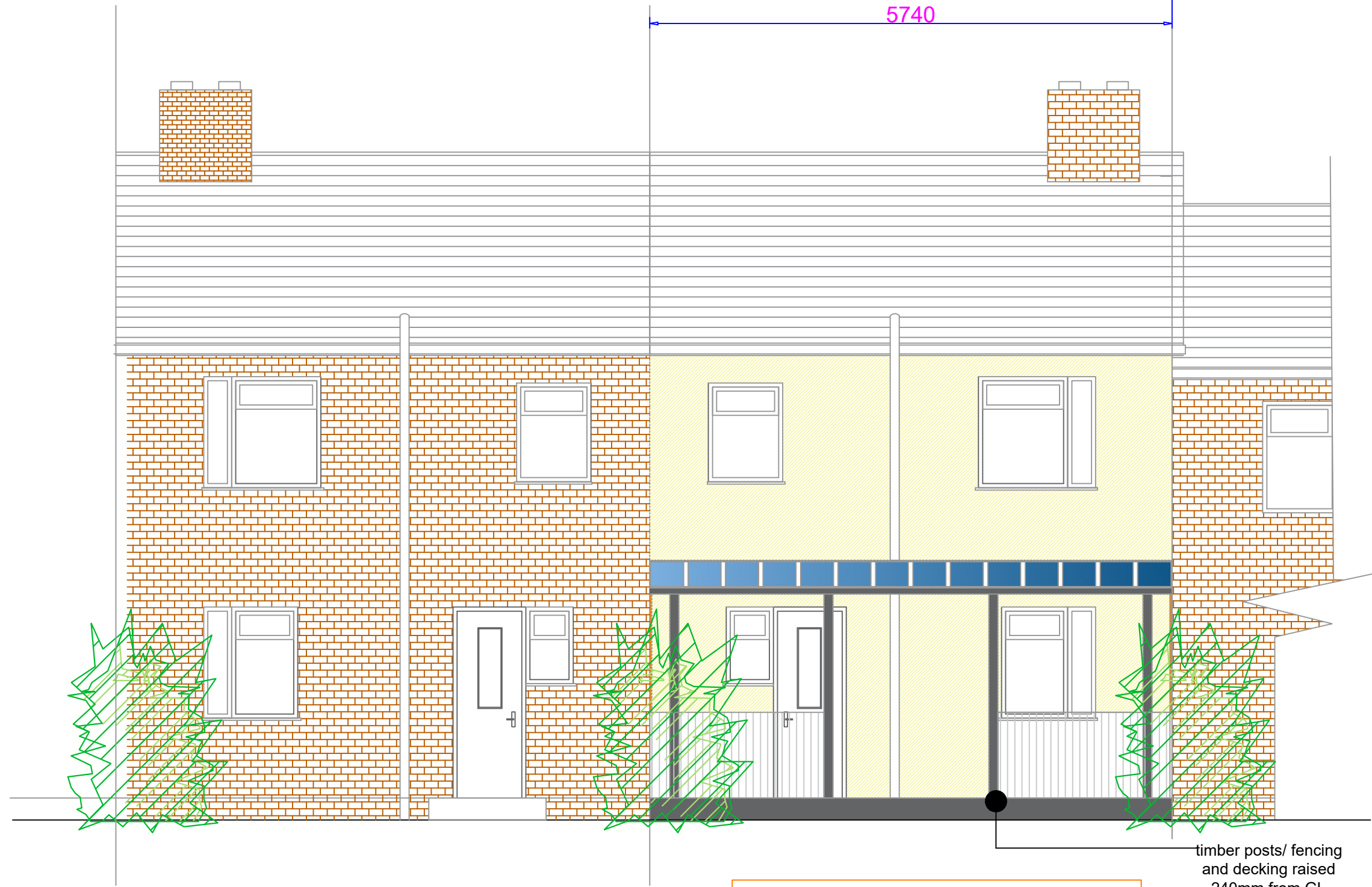
REAR EXTENSION AS BUILT
