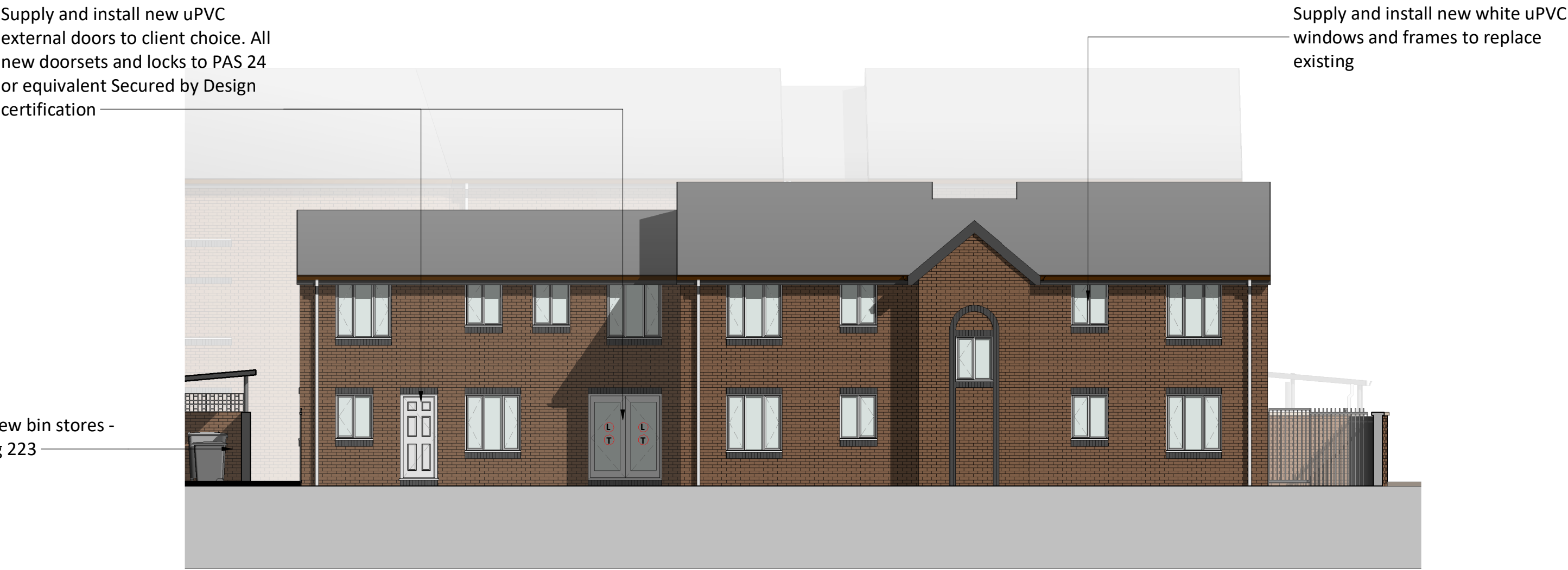
Block 1 - East (Rear) Elevation New Works 1 : 100
