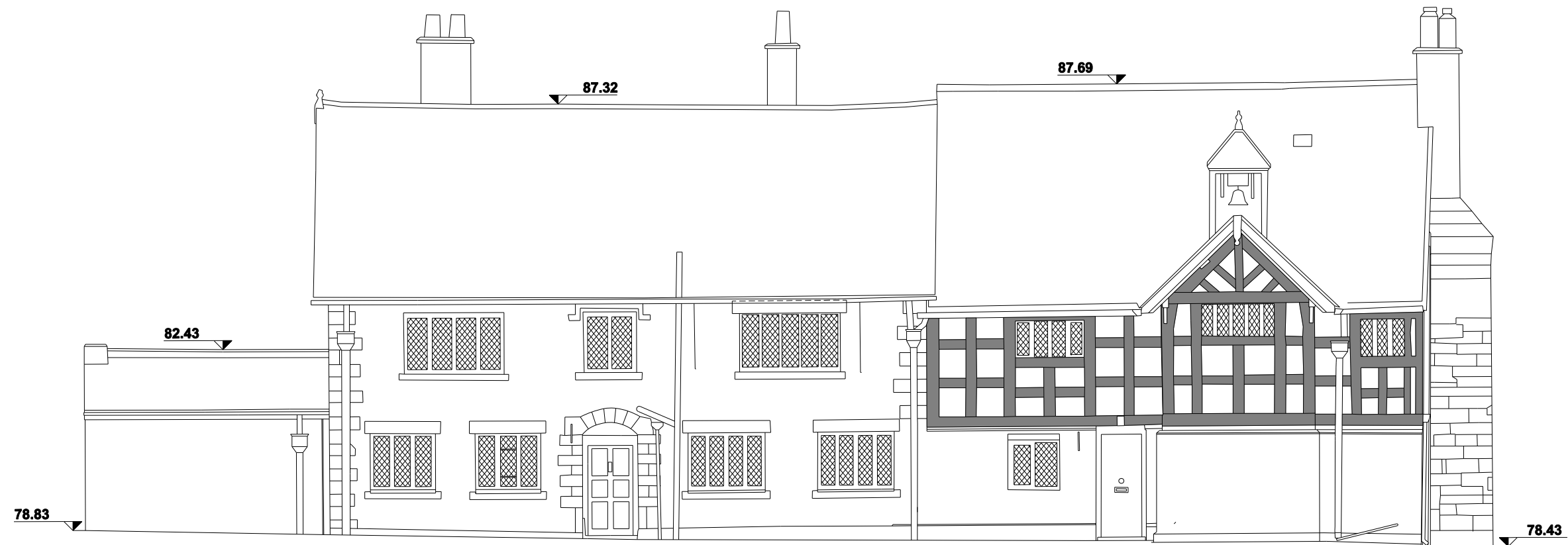
WEST ELEVATION AS EXISTING
