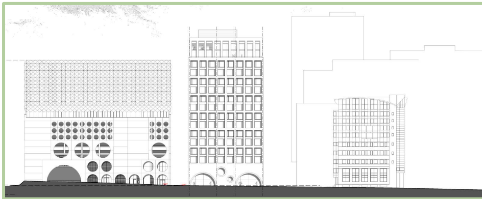
Figure 2.7 Indicative elevations to demonstrate heights at 14 storeys
