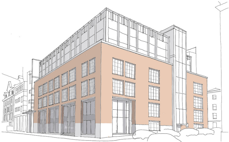
2 Crittal style windows introduced to North and West elevations
