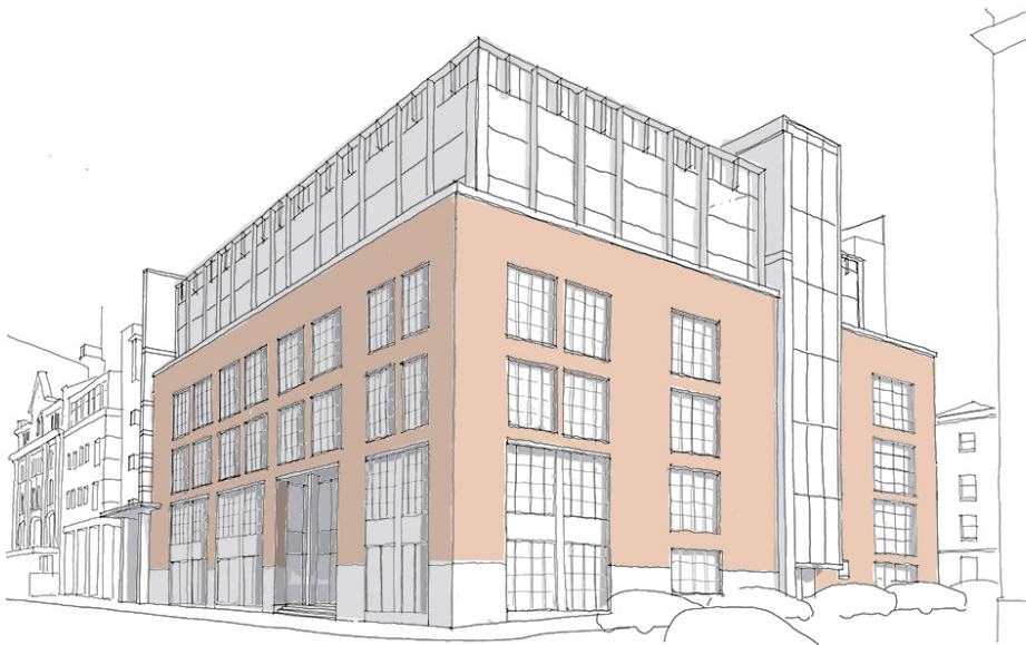
3 Ground floor recessed areas infilled with full height glazing
