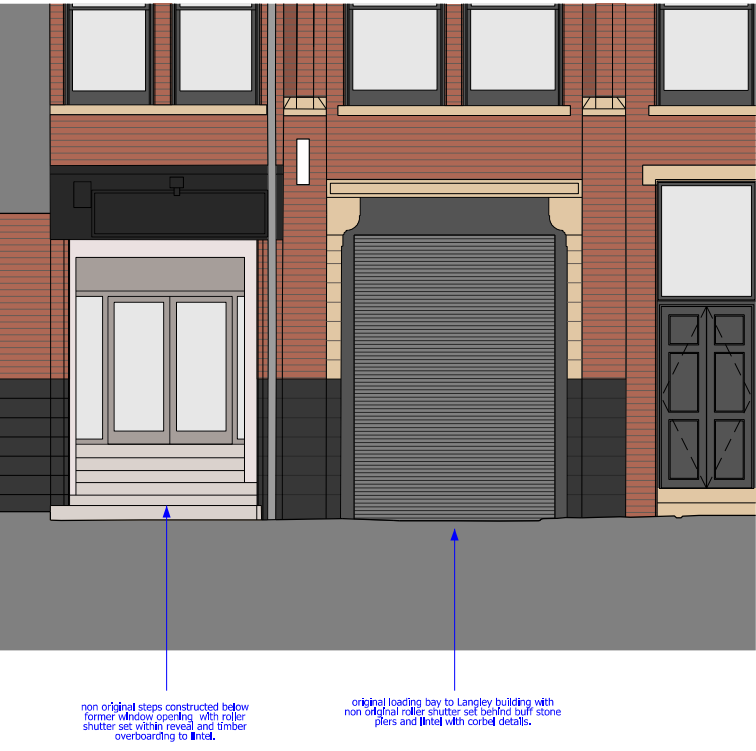
Existing Elevation - Harter Street 1:50
