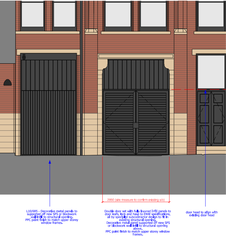
Proposed Elevation - Harter Street 1:50
