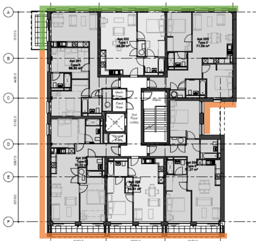
Plan showing sound insulation performance zones for facades
