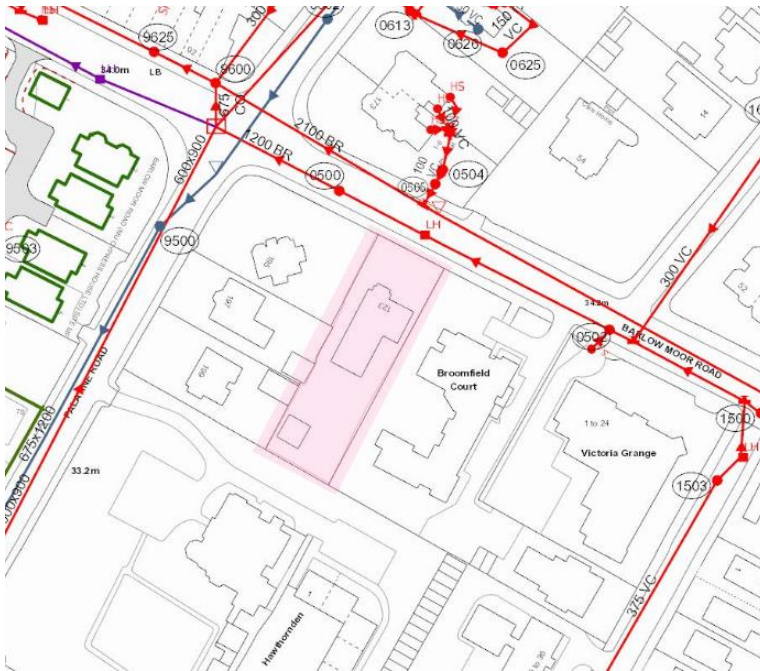
Figure 5 United Utilities Sewer Records
