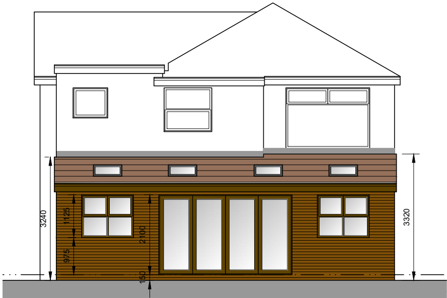
North East Facing Rear Elevation
