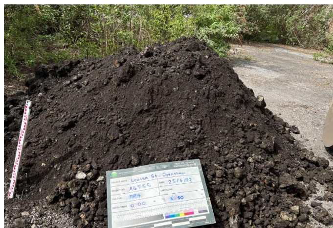
Trial Pit 4: Overview of excavated soils
