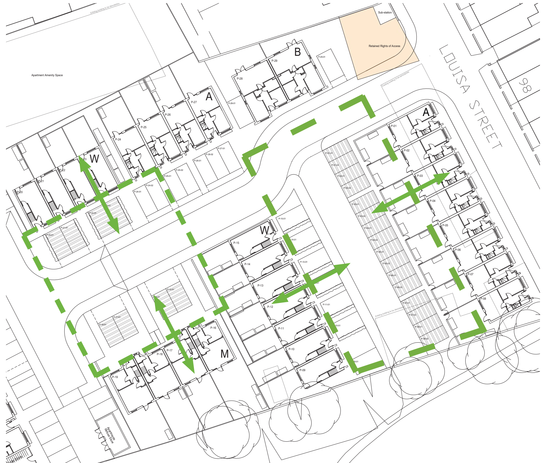
Highlighting opening of grid to create courtyards.
