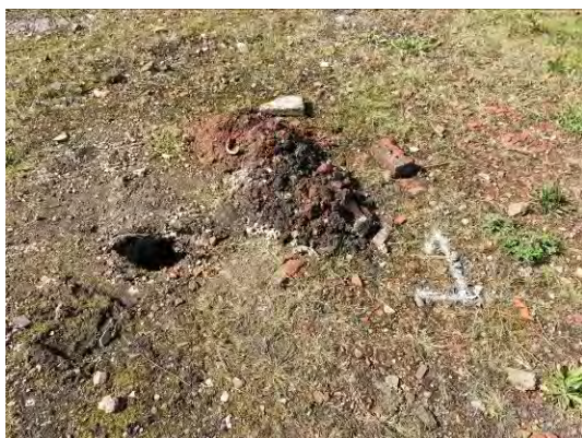
Photo E – Typical made ground spoil. WS01.
