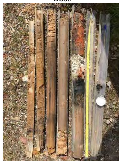
Photo F – Typical window sample core. Made ground to 0.7m clay to 1.9m and clayey sand to 4.0m. (WS07)
