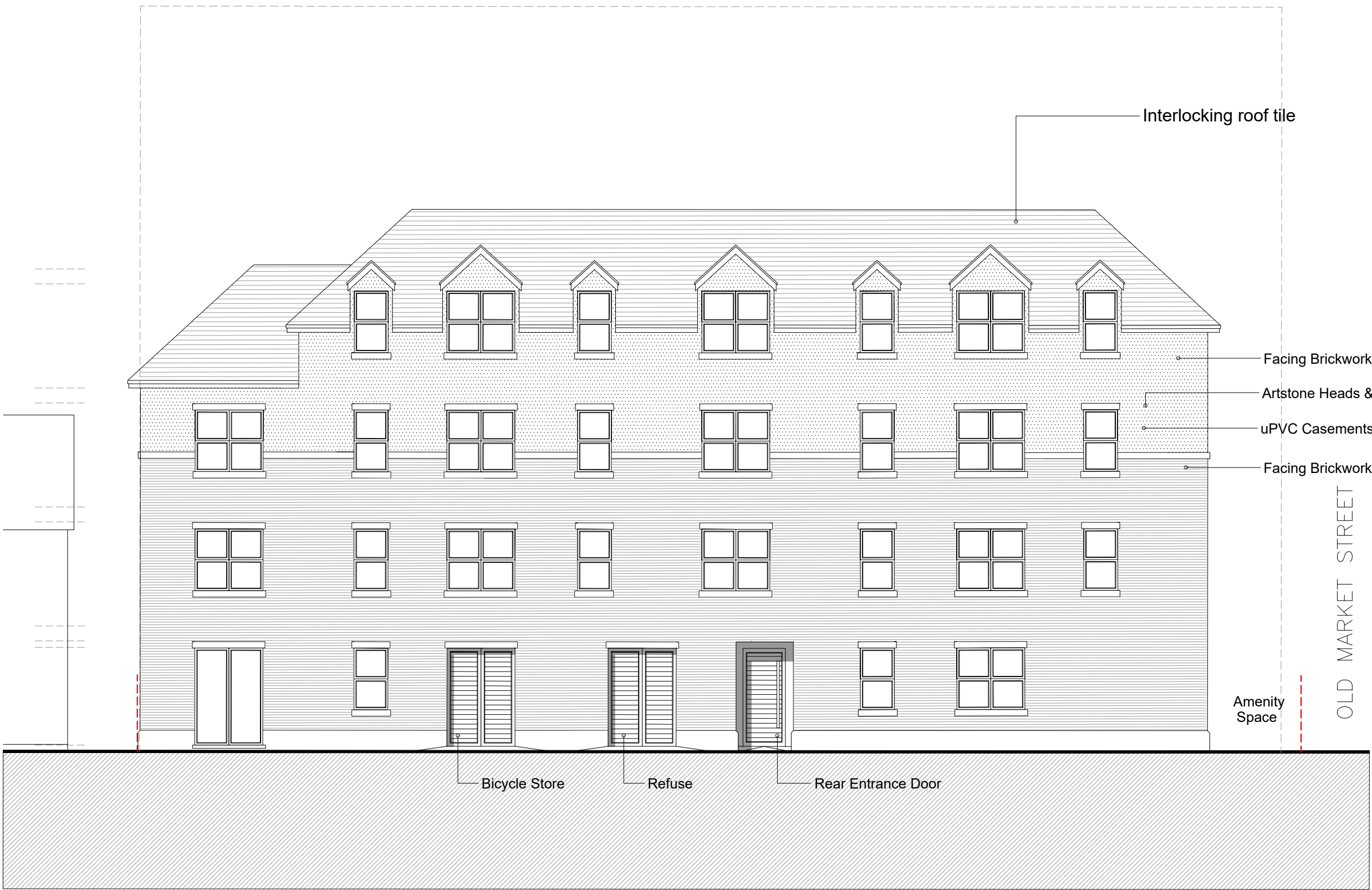
PROPOSED ELEVATION (C) EAST - FACING PARKING AREA 1:100
