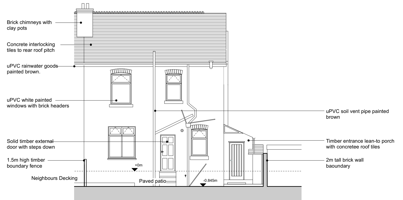
Existing East Elevation (Rear) 1:100
