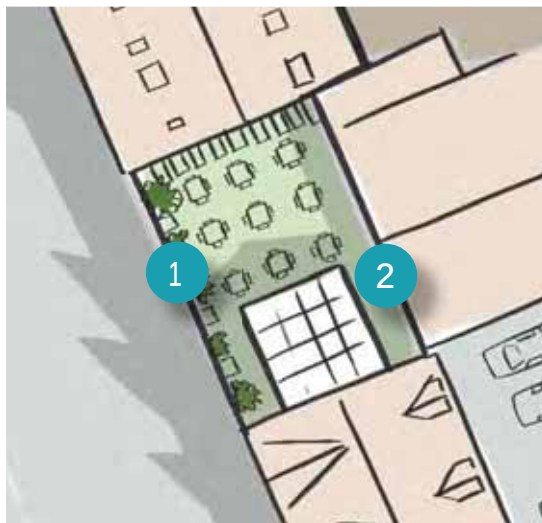
Location plan showing the unattended logger and short-term attended measurement positions
