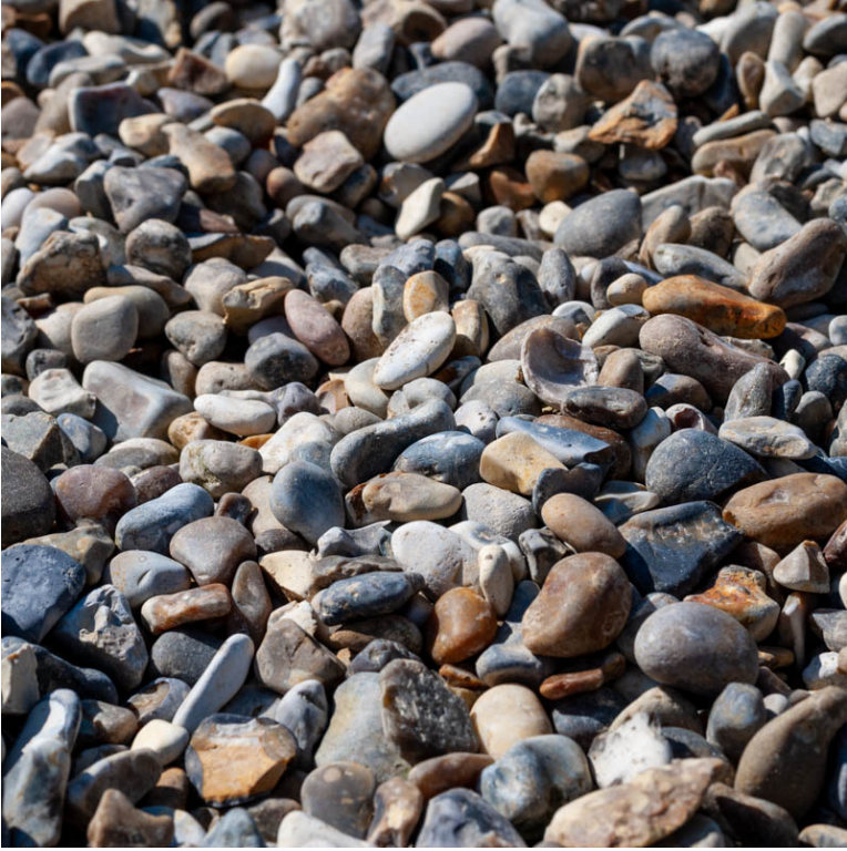
Decorative Gravel - 20mm - adjacent to facade where deeper build up can't be achieved
