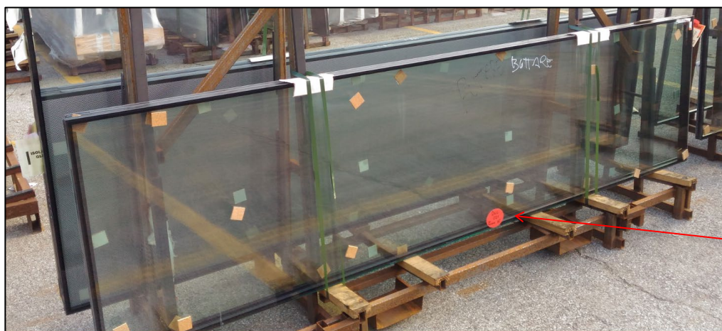
Red label to identify non-compliant material
