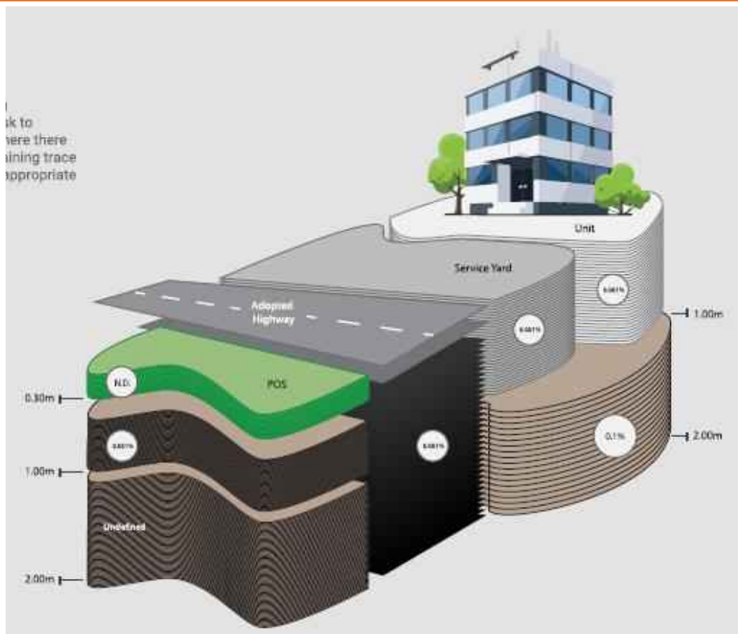
FIGURE 4.1 ASBESTOS RISK MITIGATION CONCEPTUAL SITE MODEL
