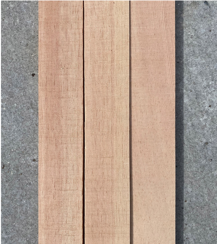
Quarter sawn Douglas Fir timber samples prior to the application of a protective topcoat,
