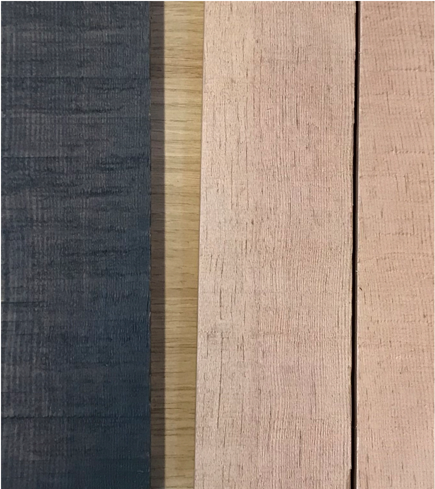
Quarter sawn Douglas Fir timber sample following the application of a protective topcoat (left),
