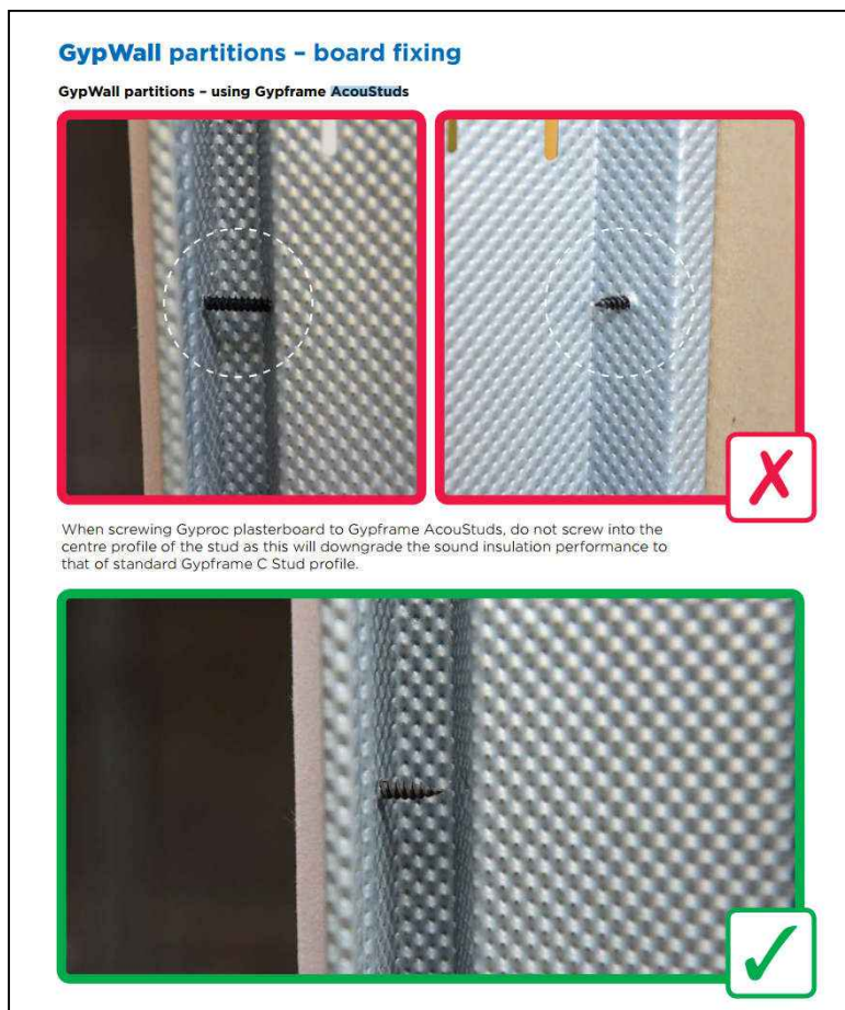
Figure 1: Plasterboard fixing to acoustic studs (© British Gypsum)
