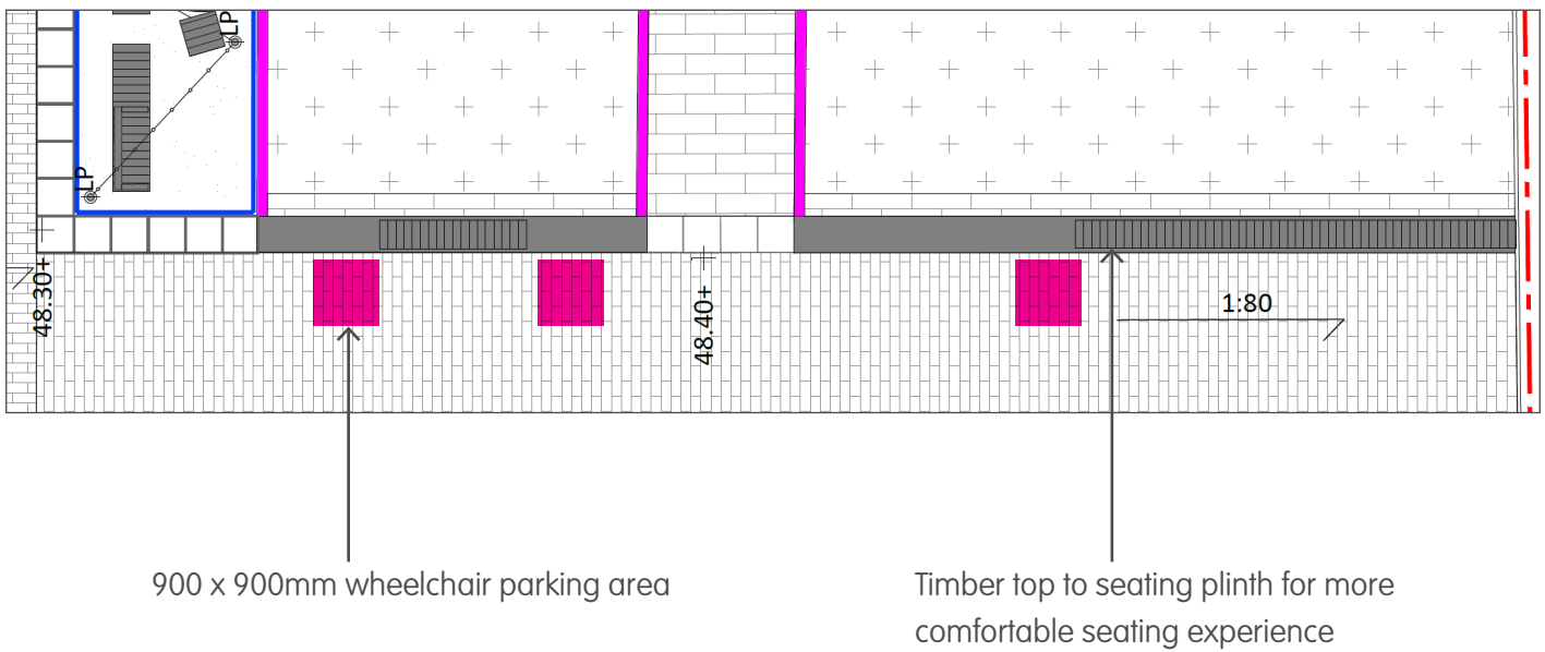
Detailed extract of seating plinth from drawing CAS-RFM-XX-L0-DR-L-19-0022-S2-P01
