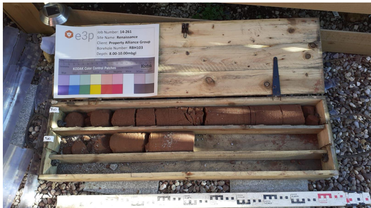
PLATE 4 RBH103 ROCK CORE (8.00 – 10.00 m bgl)
