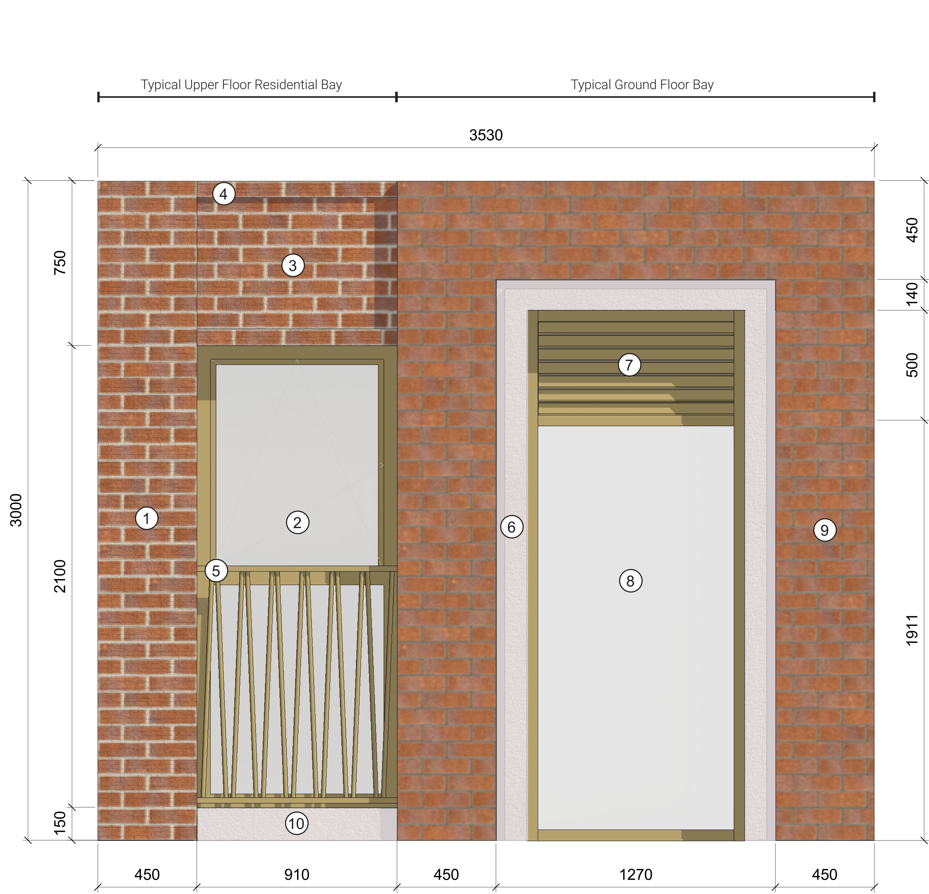
1 Mock Facade Panel Scale: 1 : 10
