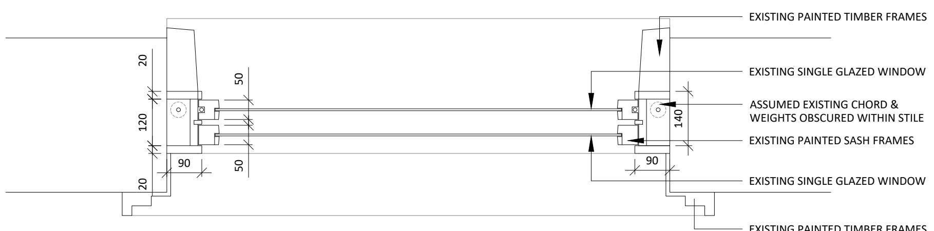
04 1st FLOOR SASH WINDOW - TYPE D 513 SCALE 1:10 EXISTING PLAN SECTION
