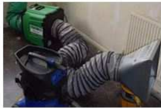
Filtrated mobile dust control unit.
