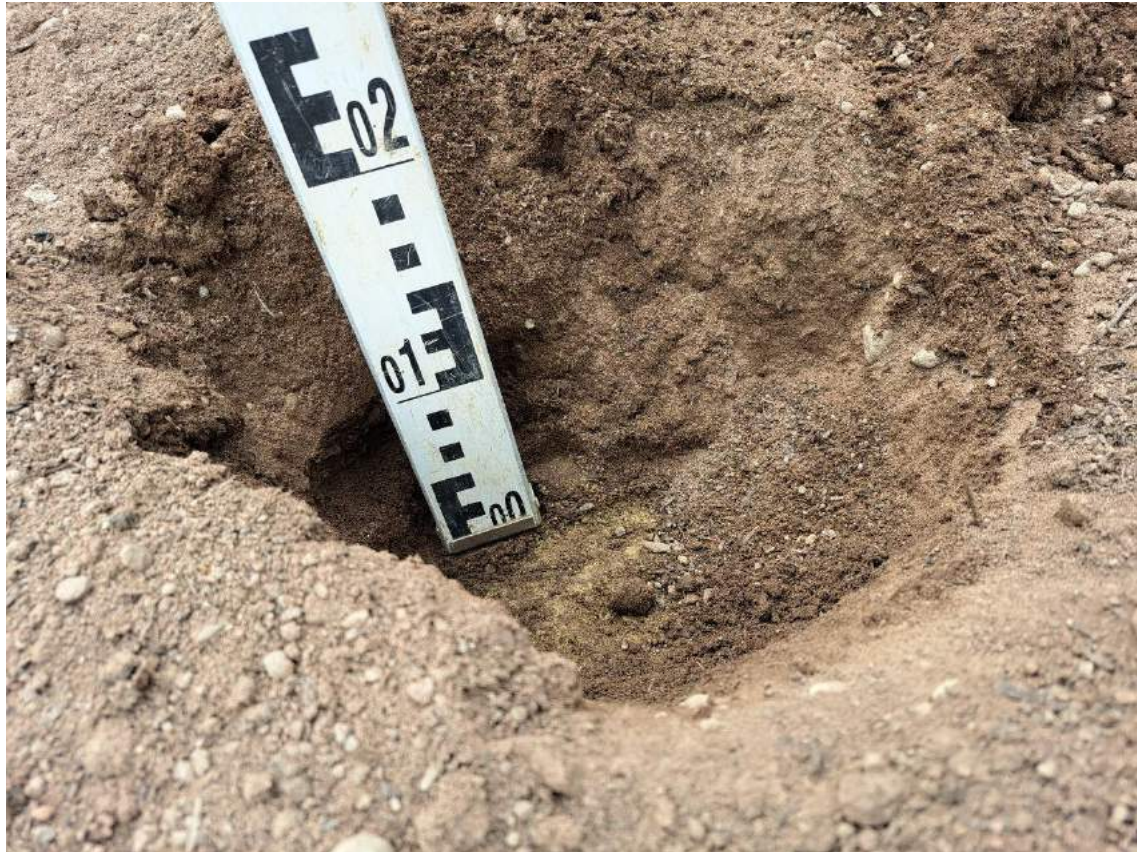
Photograph 23 200mm of imported topsoil at VP09 following import.
