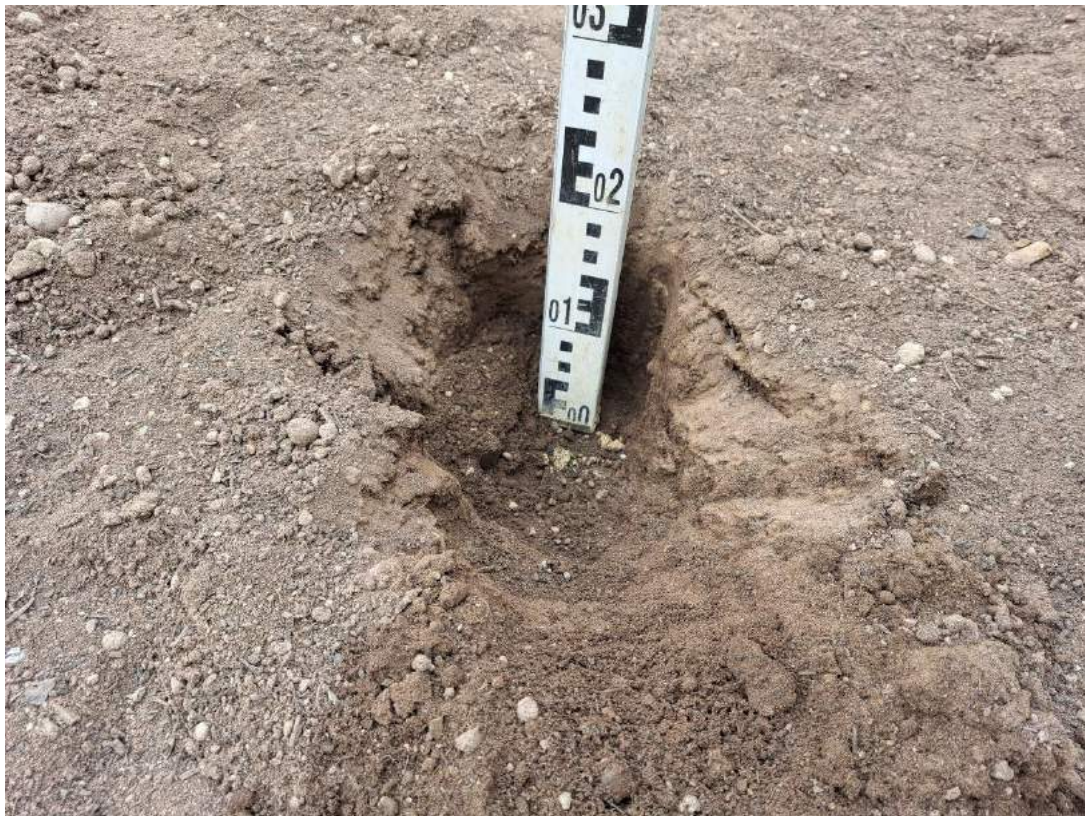
Photograph 38 200mm of imported topsoil in VP16.
