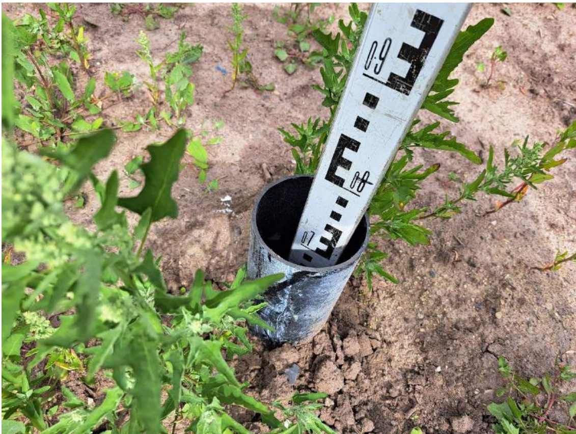
Photograph 16 300mm of topsoil overlying 300mm of subsoil emplaced in VP07.
