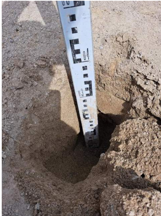
Photograph 32 250mm of subsoil emplaced in VP13.
