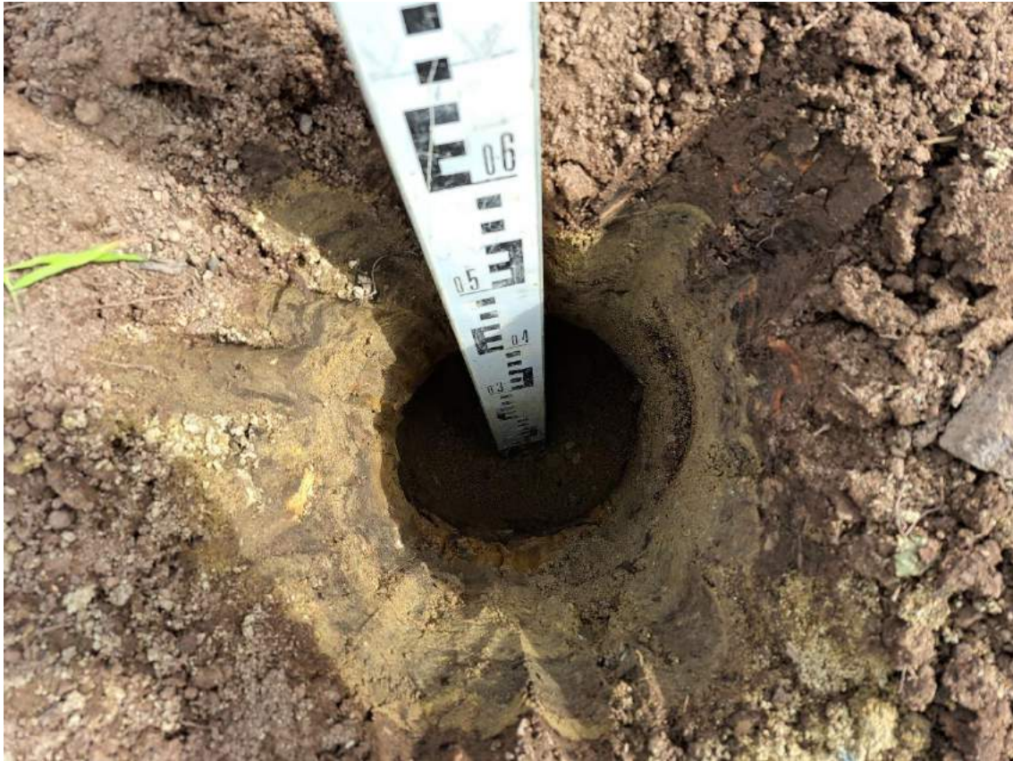
Photograph 19 Confirmation of 150mm of topsoil, 100mm of subsoil and 350mm of natural clay deposits in VP08.
