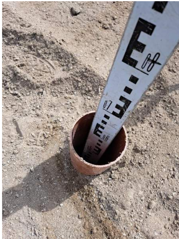
Photograph 10 450mm of subsoil emplaced in VP05 prior to importation and placement of topsoil.
