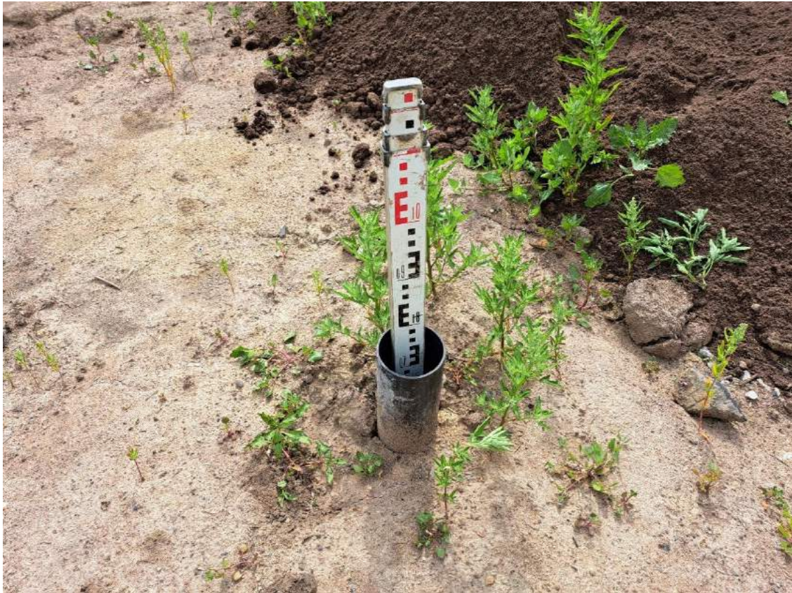
Photograph 13 250mm topsoil overlying 250mm of subsoil at VP06 prior to the importation of additional topsoil.
