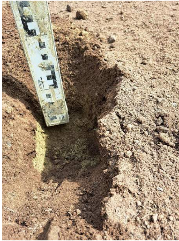
Photograph 9 Confirmation of 150mm of topsoil emplaced in VP04.
