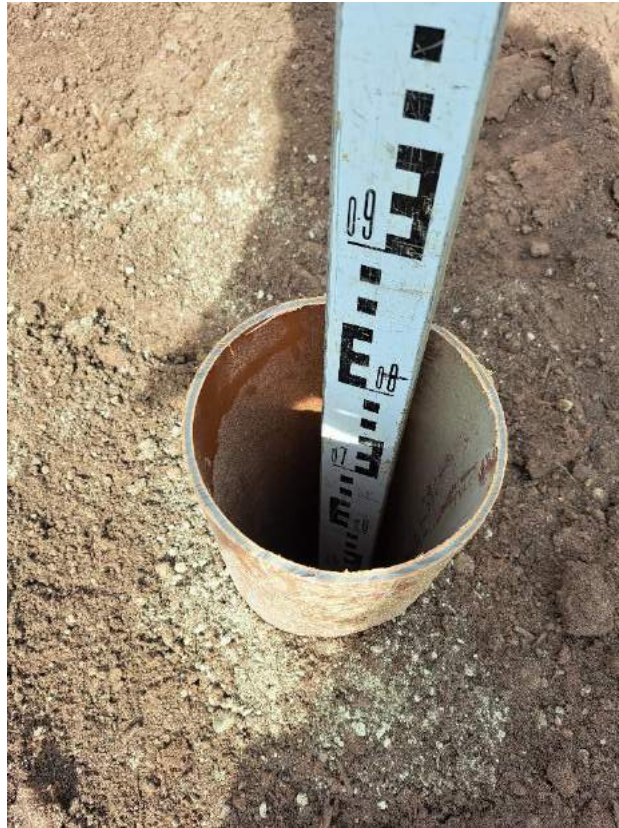
Photograph 3 250mm of topsoil and 350mm of subsoil emplaced in VP02.
