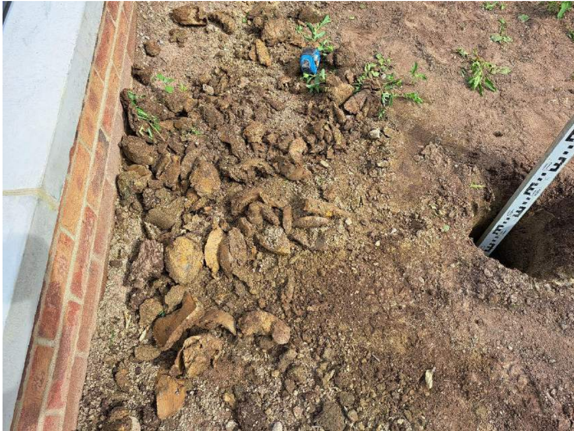
Photograph 21 Natural clay from beneath imported subsoil in VP08.
