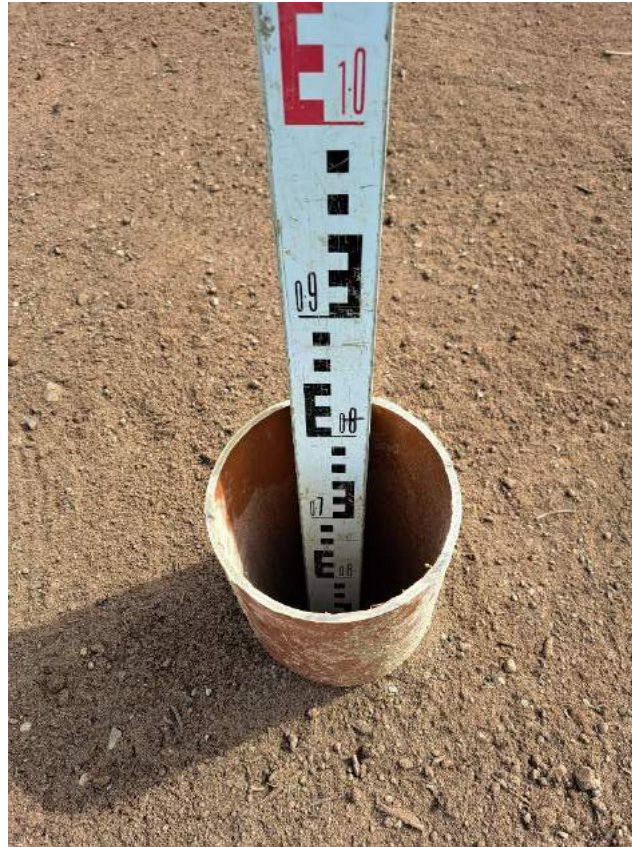
Photograph 7 150mm of topsoil overlying 450mm of subsoil in VP04.
