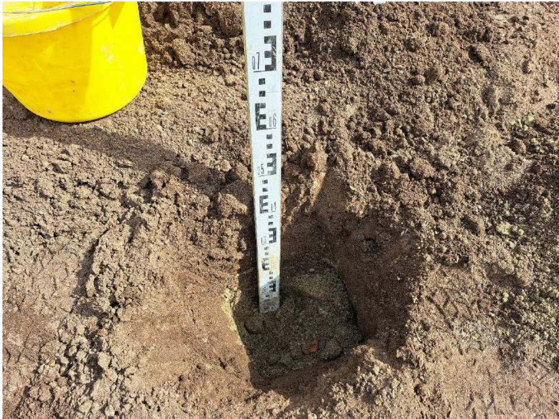
Photograph 5 300mm of topsoil overlying 250mm of subsoil emplaced in VP03.
