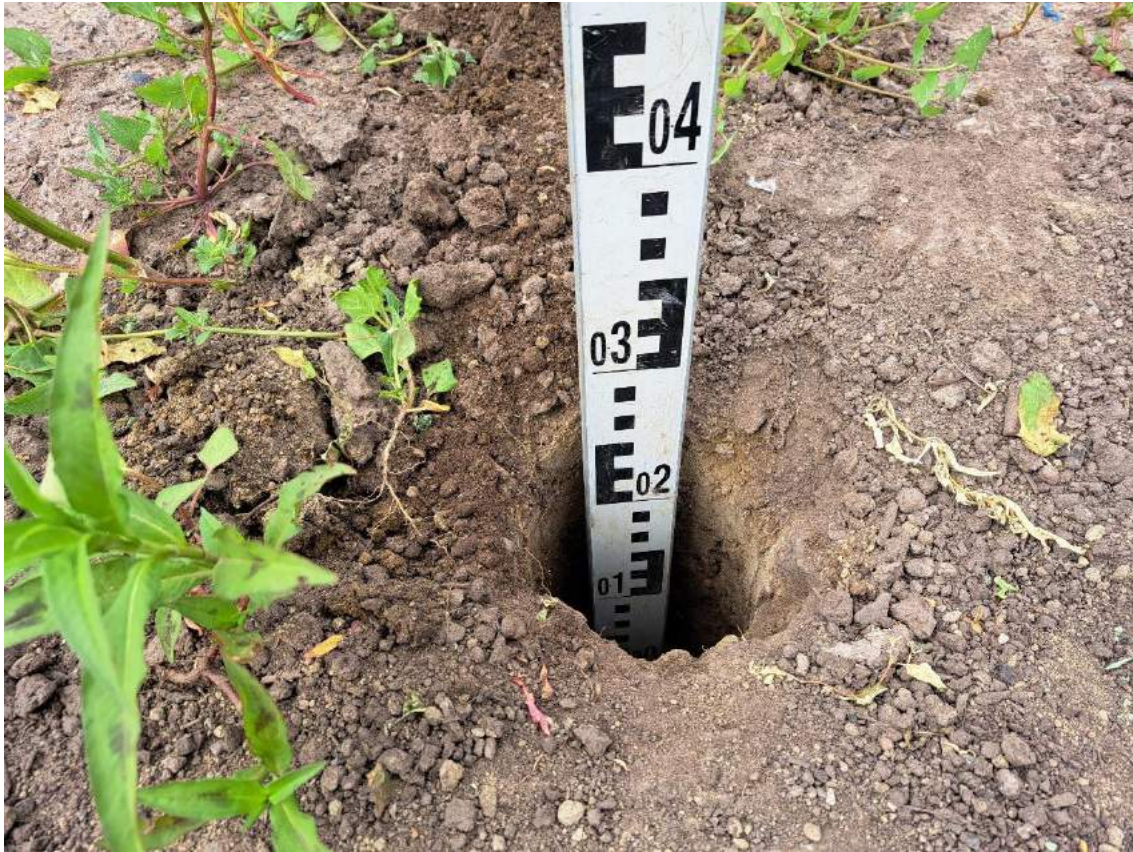
Photograph 17 Confirmation of 300mm thickness of topsoil emplaced at VP07.
