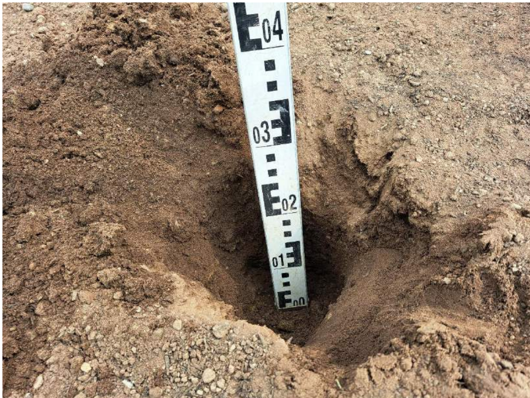
Photograph 36 300mm of imported topsoil overlying 300mm subsoil in VP15.
