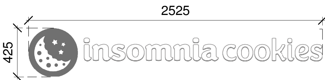
Proposed LED illuminated sign - 2 1 : 20 Internally illuminated aluminium anodised silver letters with white semi-transparent Perspex on the front faces
