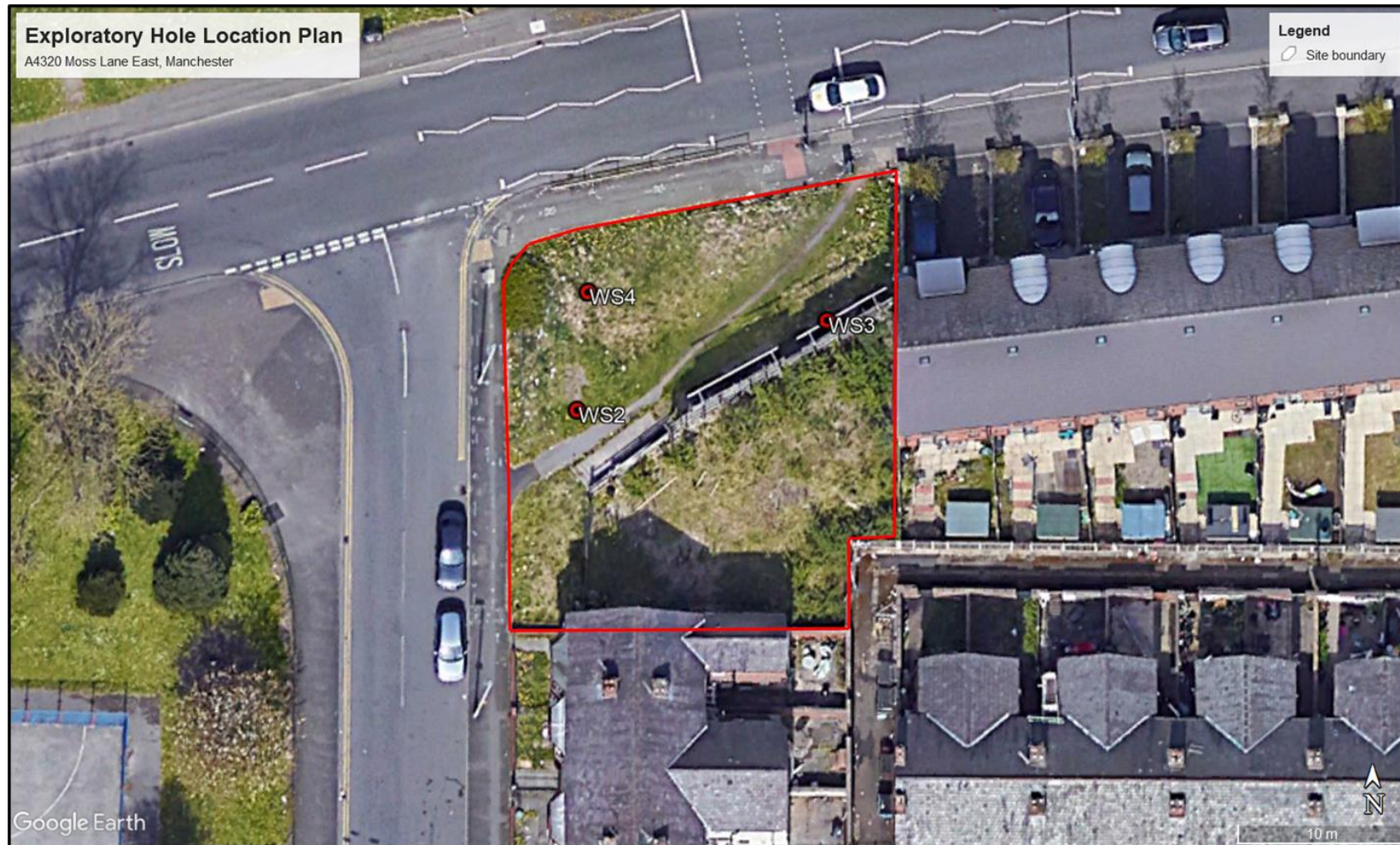
Figure 3: EEG Exploratory Hole Locations - WS Boreholes
