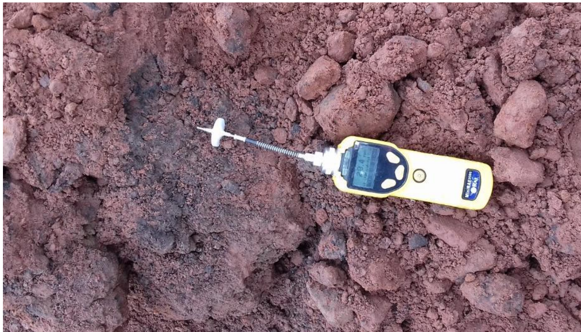
PLATE 4 – PID MONITORING OF CONTAMINATED MATERIAL
