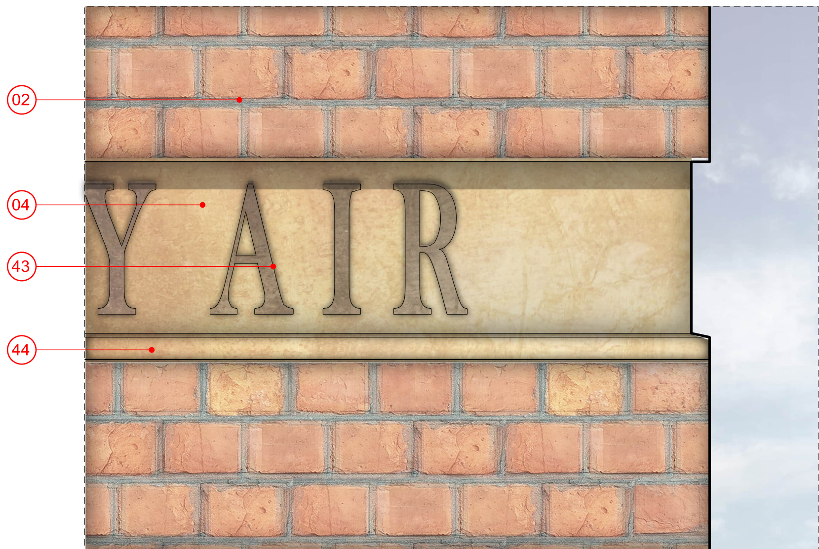
05 Bronze Inlay Text and Recess Corner Detail - PROPOSED 1:5
