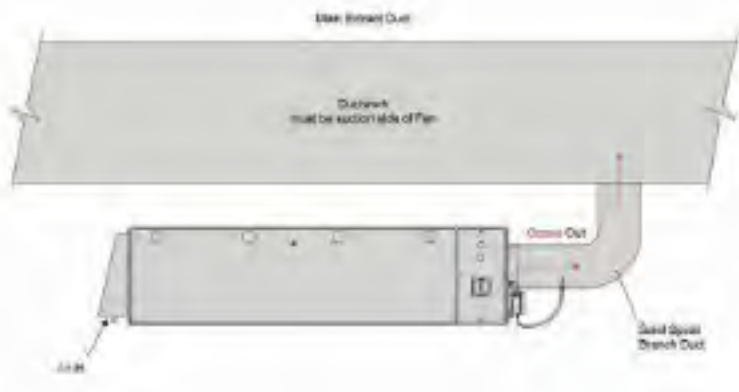
Figure 24 - UV-O 1000 Installation Schematic
