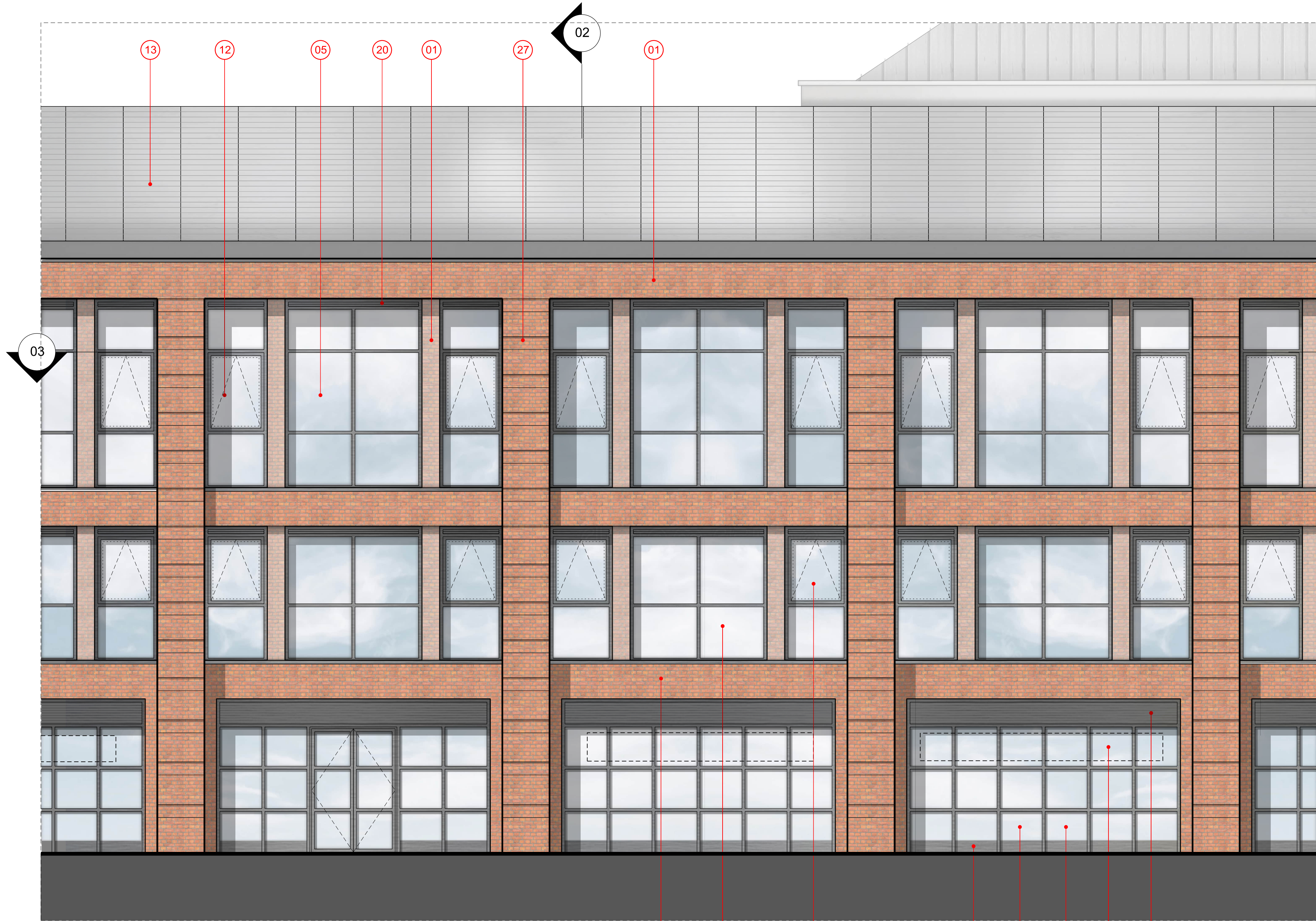
01 Typical Bay & Gable Junction Elevation - PROPOSED 1:50
