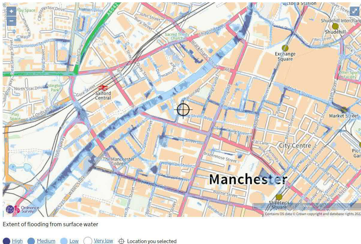
Figure 5-2 - GOV.UK's Long Term Flood Risk Map for Surface Water Flooding Extract
