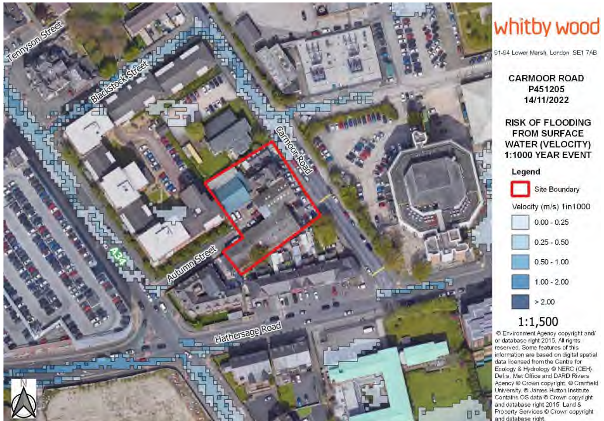
FIGURE 5 - SURFACE WATER FLOOD VELOCITY (1IN1000 YEAR EVENT)
