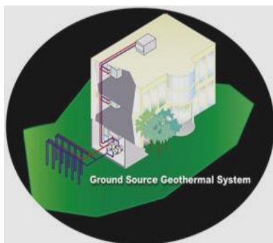
Ground Source Heat Pump Installation
