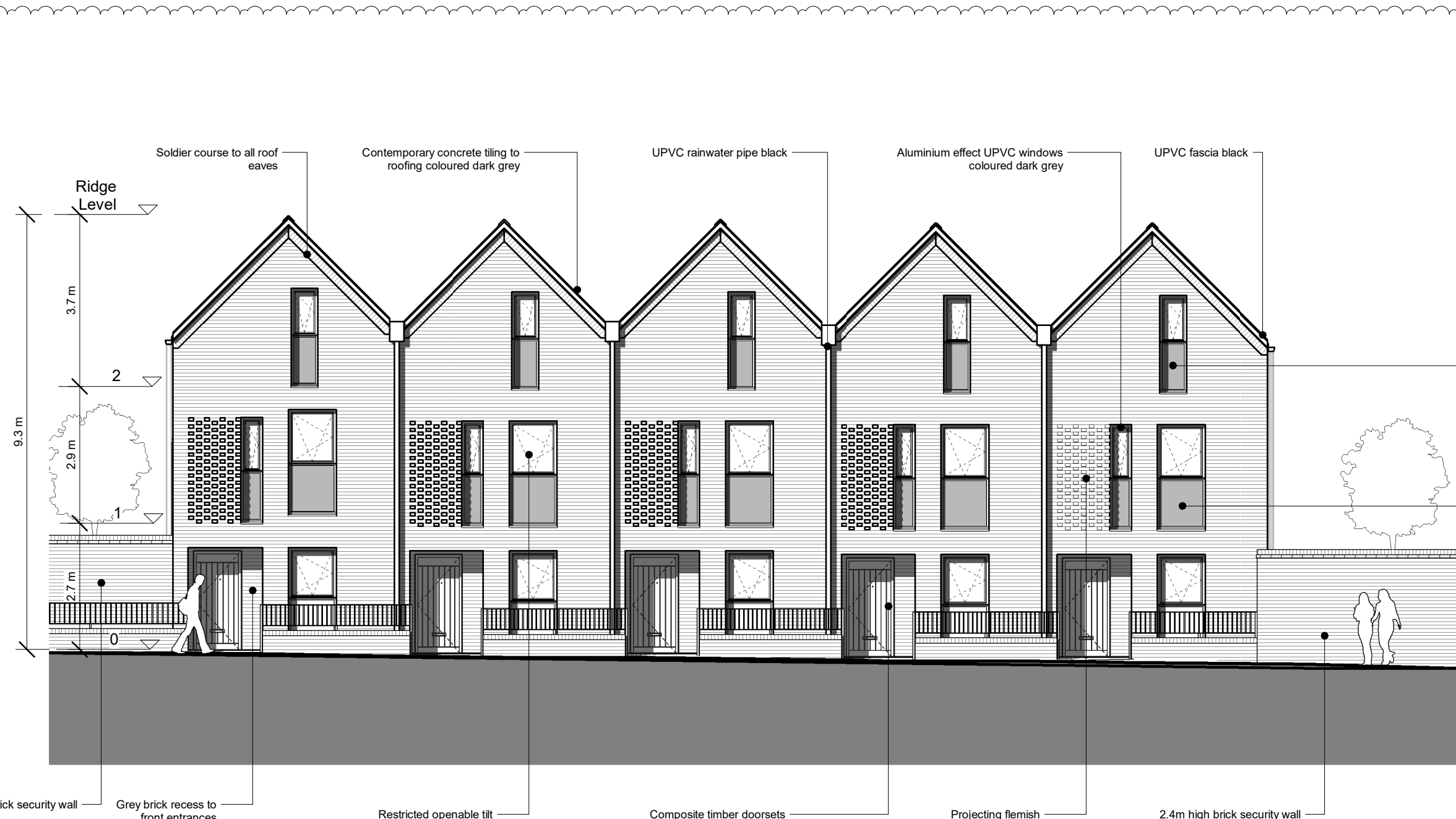
1 Building 5 - House Type 1 and 3 Proposed North Elevation 1:100
