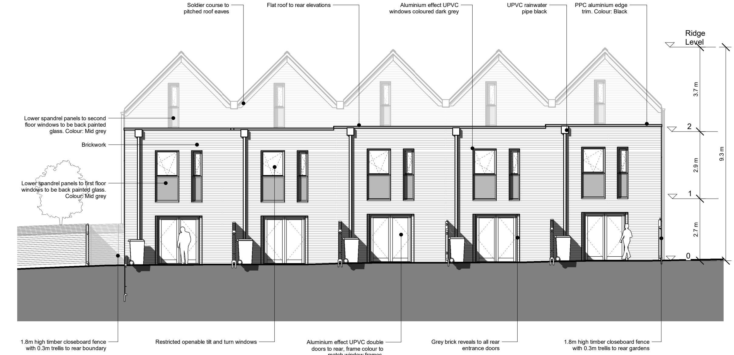
3 Building 5 - House Type 1 and 3 Proposed South Elevation 1:100
