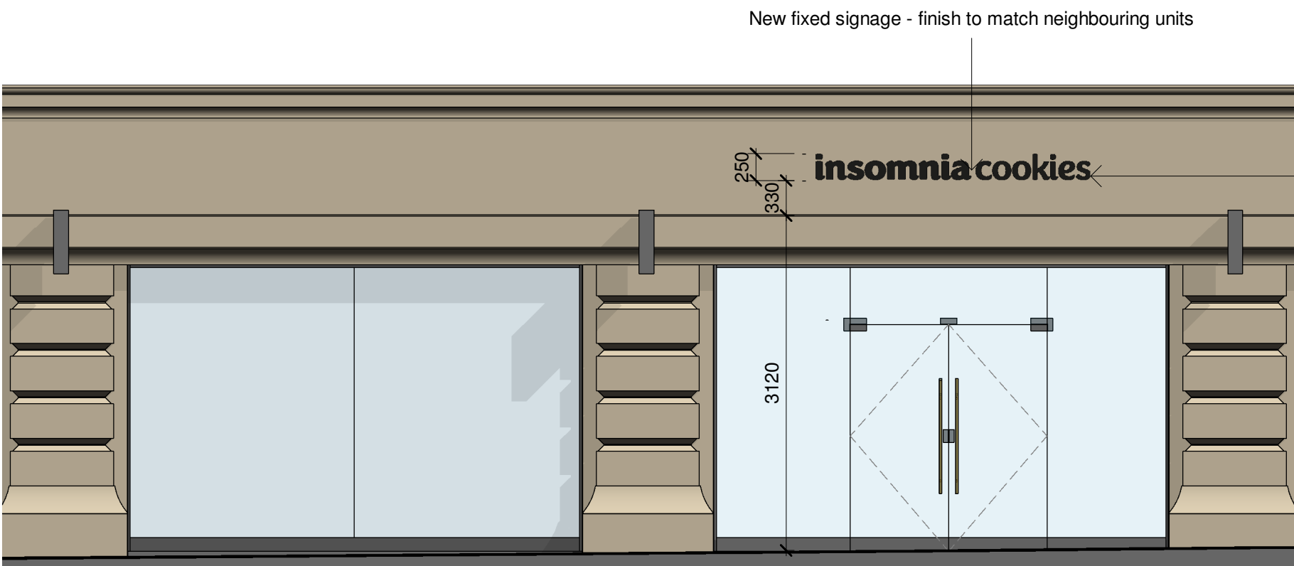
External elevation - proposed 1 : 50
