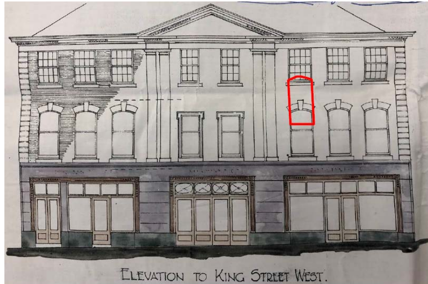
Figure 8: 1926 proposed elevation on King Street West. The red outline illustrates the original location of the windows
