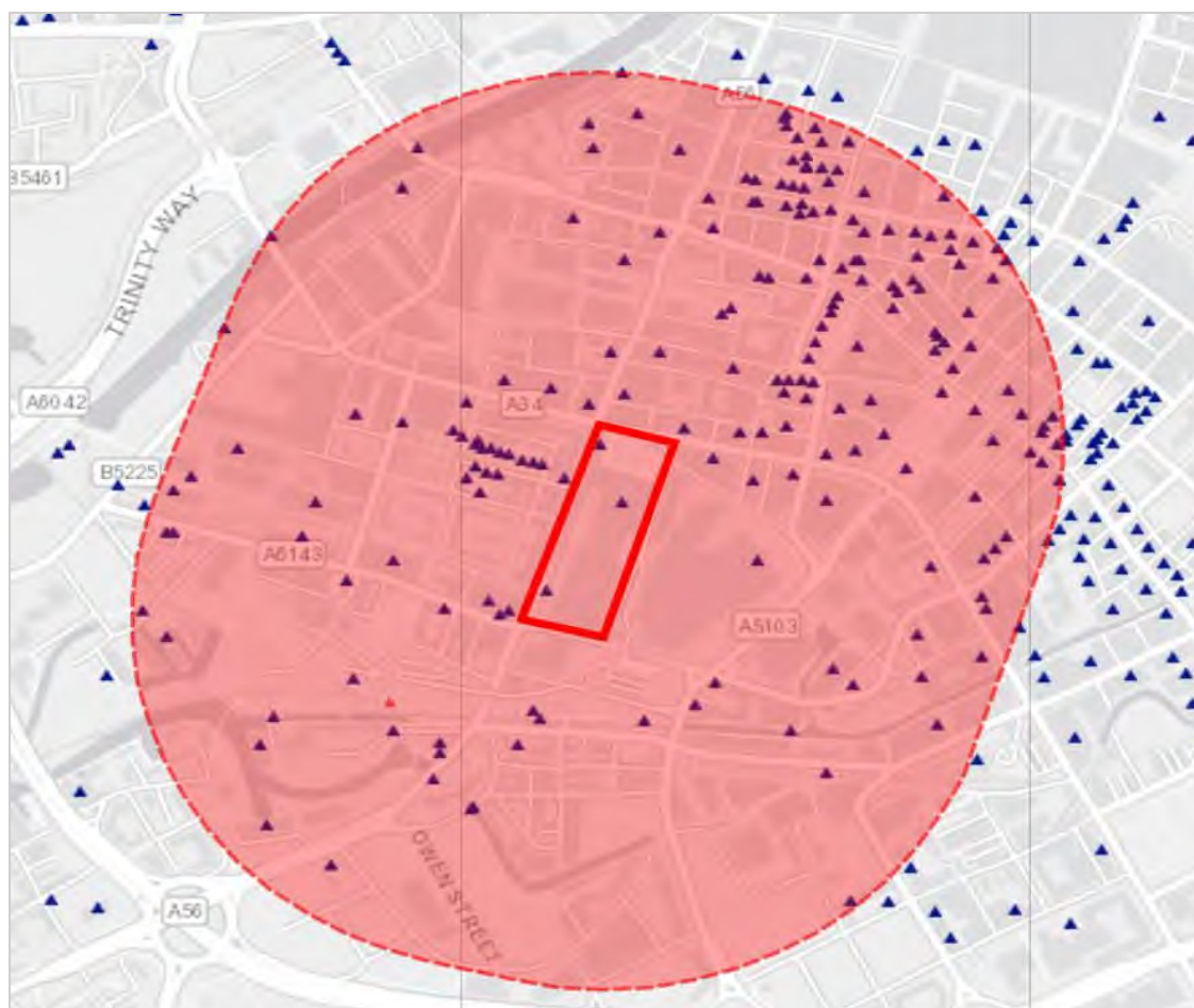
Figure 5: Scoping exercise, listed buildings (identified by blue triangles) within a 500m radius around the subject site (identified by red line). Extent of 500m radius shaded red. Source: Historic England NHLE.
