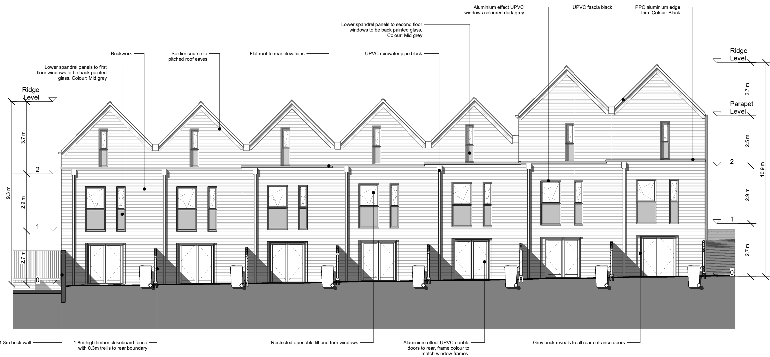
3 Building 2 - House Type 1 and 3 Proposed South Elevation 1:100
