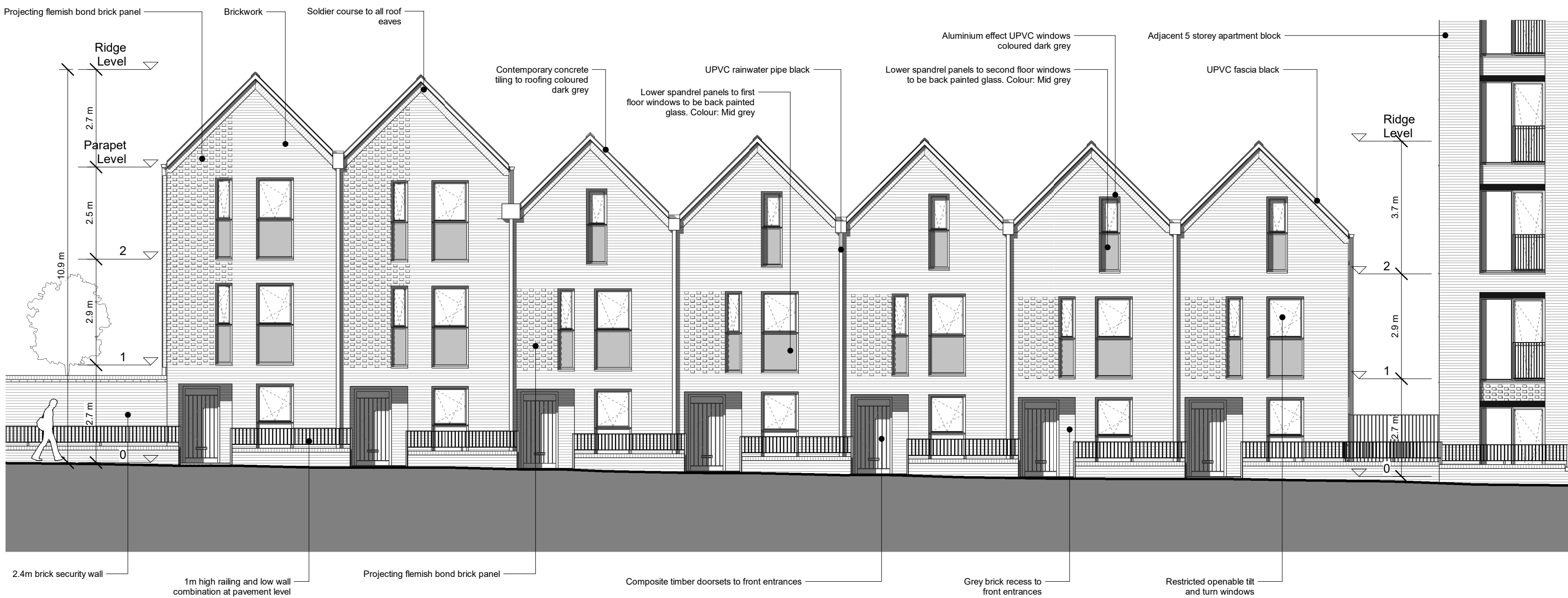
1 Building 2 - House Type 1 and 3 Proposed North Elevation 1:100
