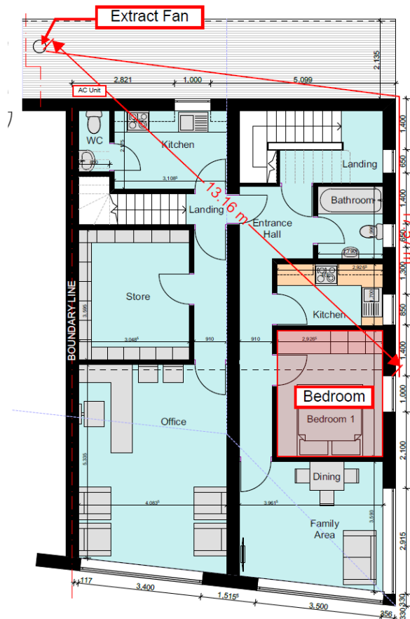
Figure 3 Proposed first floor showing bedroom in relation to extract duct and AC condenser unit
