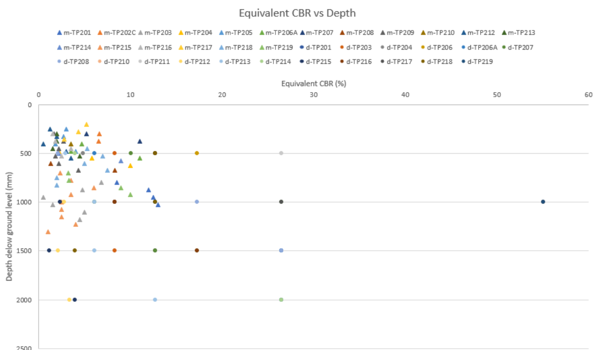
Figure 10: Equivalent CBR vs depth based on in-situ mexeprobe and DCP results
