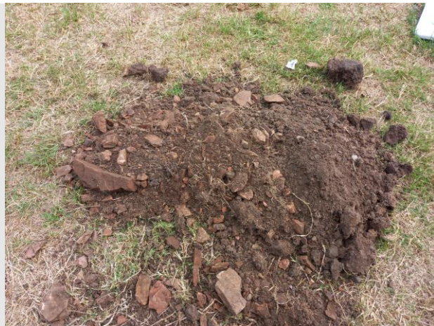
Photo 21: Backfill material containing soil
