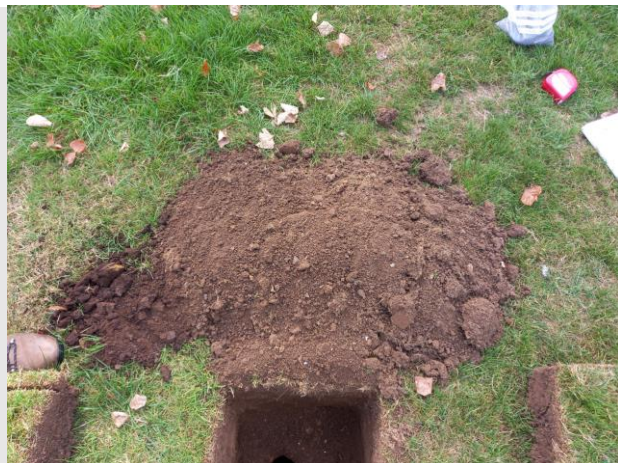
Photo 17: TP2 showing gradual transition from topsoil to darker subsoil
