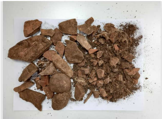
Photo 22: Backfill material sample containing soil
