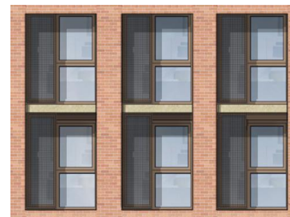
Typical Facade Purge Panels
